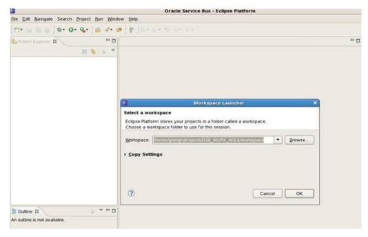
To summarize, RSB\_WORK\_AREA is the location where jars are copied to and from the RSB builder location and OSB\_WORK\_AREA is the location where jars are imported as OSB projects and are worked upon.
